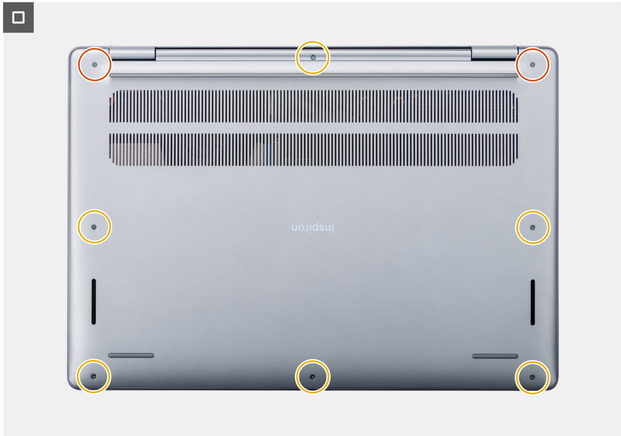
Figure 9. Installing the base cover
