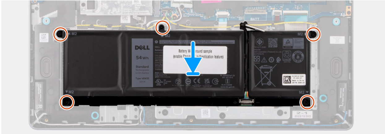
Figure 23. Installing the battery
