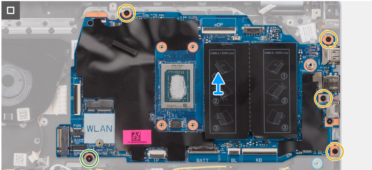
Figure 42. Removing the system board
